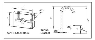
In order to check all relevant dimensions and to test if all parts can be assembled you have to make an inspection plan of the steel block (part 1) and the bracket (part 2).
